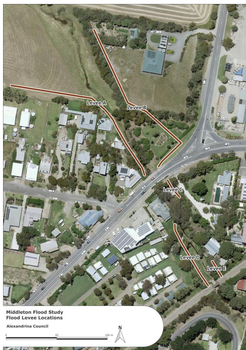
Figure 7-3: Approximate locations of potential flood levees
